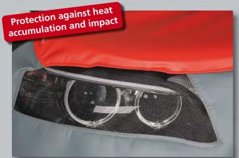
The special **red sandwich paddings** (five layers with sheet **steel reinforcement**) effectively protect the technician in the case of unintended activation of the pedestrian safety device.
